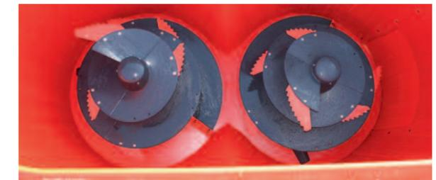
*The polygonal shape of the hopper acts as a brake, holding the material for longer to increase the rate of chopping. Details such as the pitch of the auger coils and positions of knives on the auger all contribute to more efficient processing of long fibre.*
